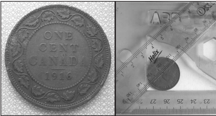
The design of this Canadian large cent makes it an ideal choice for a double-sided coin ring. It's a cinch to determine a coin's exact center with the aid of an easily assembled plastic jig.
