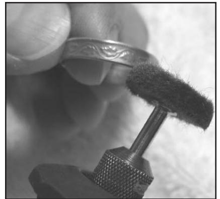
Final polishing with a felt disk, tripoli, and jeweler’s rouge gives the ring a rich, lustrous look.
