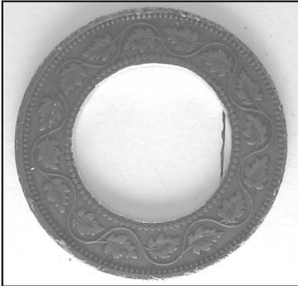
With the center carefully removed by repeated drilling and burring, the coin now resembles a washer.
